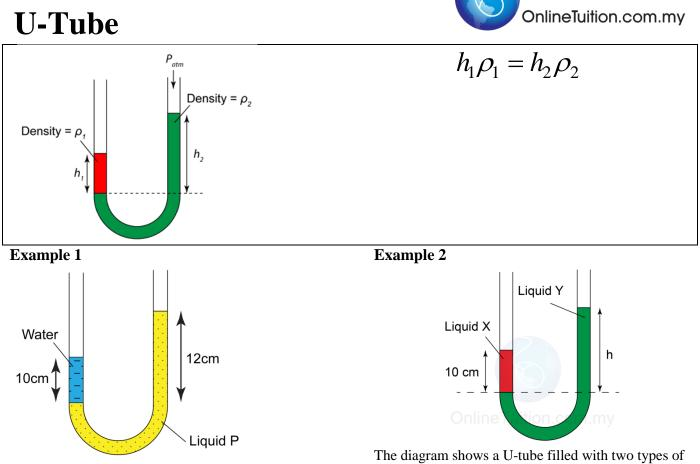
Figure above shows a U-tube filled with water and liquid P. Liquid P is insoluble in water. Given that the density of water is 1000kg/m<sup>3</sup>, find the density of liquid P. The diagram shows a U-tube filled with two types of liquid, X and Y which are not mixable. If the density of liquid X and liquid Y are 1200 kg/m<sup>3</sup> and 800 kg/m<sup>3</sup> respectively, find the value of h.
